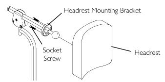
FIGURE 9.2 Replacing Headrest
